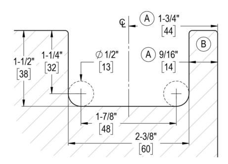
Dimension(s) can be increased as needed to accommodate projections
